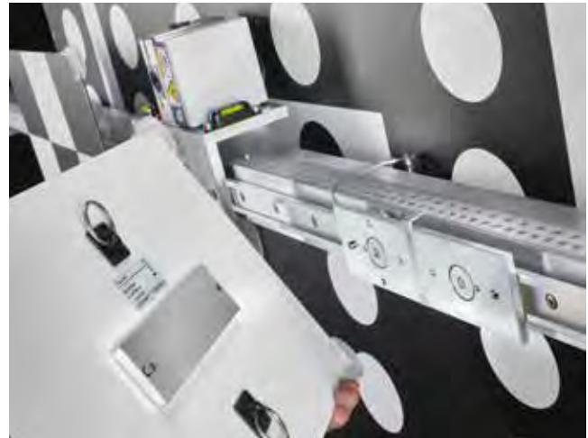
Attaching calibration targets to the sliders of the BBFAS 1415 calibration beam by means of magnetic adapters
